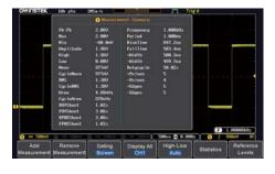
display screen. Users can also select to show all parameters if the preset eight sets are insufficient. Once the selection is made, all 36 measurement parameters will be shown on the center of the display screen. This is a very convenient measurement tool for students writing dissertations or engineers writing reports.
